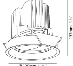
Ø 125mm 4 <sup>15</sup>/<sub>16</sub>" Ø 139mm 5 <sup>1</sup>/<sub>2</sub>"
